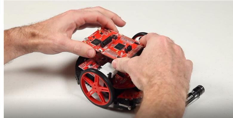
Figure 1 Dis-assembly of TI-LaunchPad from the robot
