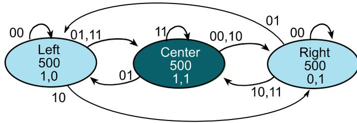
Figure 2. Moore FSM state graph to implement line following. The time in each state is shown in 1ms units.
