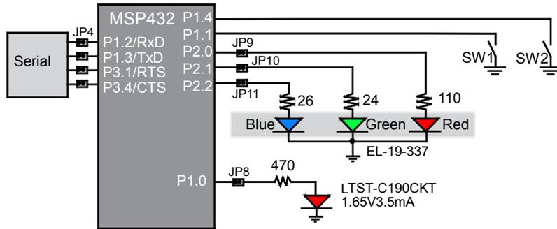
Figure 5 P1.4 is the left sensor, P1.1 is the right sensor, P2.1 is the left motor P2.0 is the right motor.
