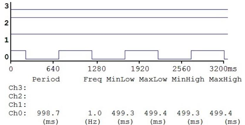
Figure 6. Logic analyzer trace showing the oscillation on the right wheel Channel 0 is 1 Hz and has a 50% duty cycle.
