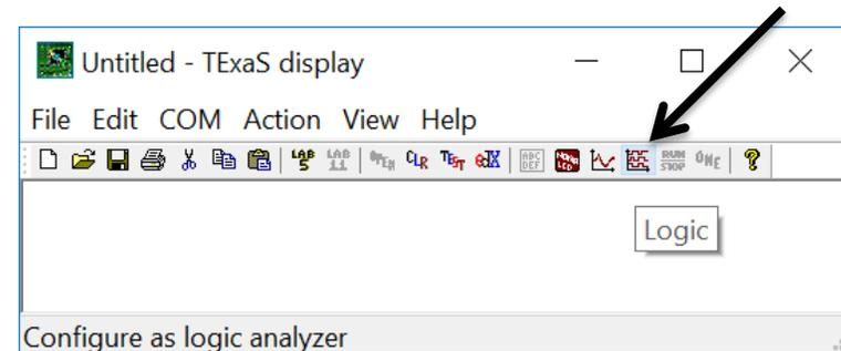
The logic analyzer always sends 7 bits at 10 kHz, but you can choose which ones to plot on the display. Execute **View -> Logic Analyzer Configuration** and disable pins 6,5,3,2 (because they have no value in this example). Specify a rising edge trigger in bit 0. The analyzer takes multiple readings and lines up the traces using the trigger. Using a trigger means one of the traces will not jitter around if the data are rapidly changing.
