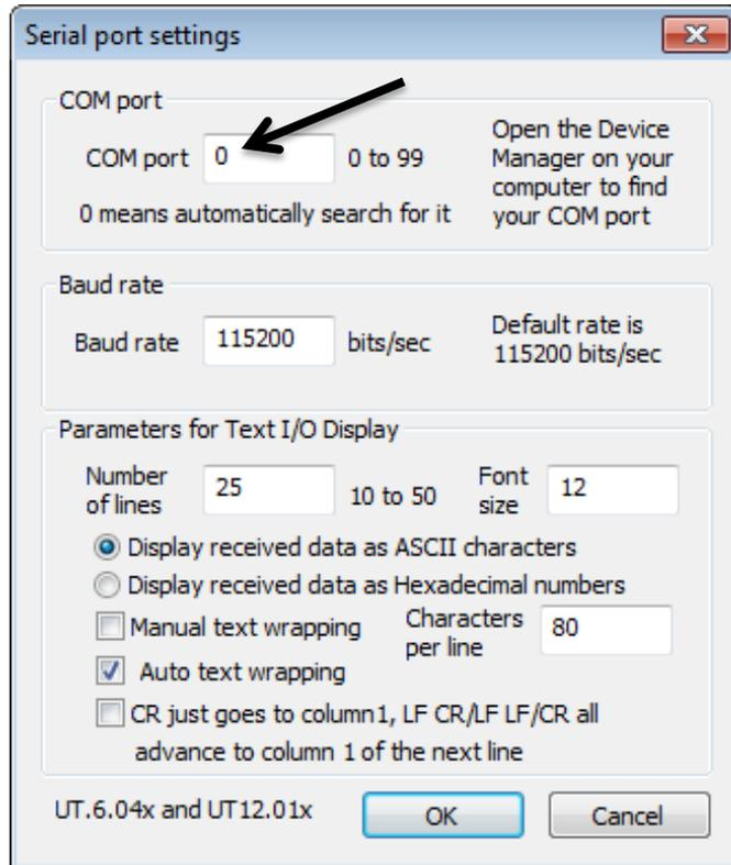
To connect **TExaSdisplay** with the MSP432 serial port, you click the **Open** tool button or execute the command **COM -> Open Port (F4)**. On this computer, the MSP432 LaunchPad was found as COM7.
